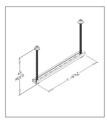
**ASP1806CR Cable Trapeze** – Is designed to be easily attached to any ASP equipment or work platform to support cable runs. Each Cable Trapeze attaches directly to the platforms by bolting through the grating floor using allthread rods with washers and nuts provided. Each Cable Trapeze can be manufactured in various sizes.
