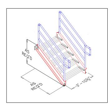
ASP4860ST – Stairs – Is designed to attach directly to any ASP platform or existing platform where stair access is required. Angle brackets used to attach top of stairs to platform. Width varies to fit into size of opening in either a guardrail or handrail.
