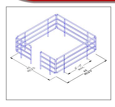
**ASP4BHR** – **Four Bar Handrail** – Is designed to be easily attached to any ASP equipment or work platform. Handrails are attached directly to the platforms by utilizing a receiver that can be welded directly to the platform or can be bolted through the grating floor using angle brackets. Handrails can be manufactured to fit any size platform.
