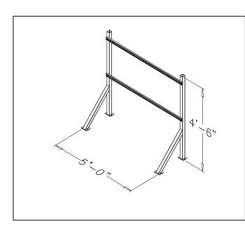
**ASP5460L Power/Telco Rack** – Is designed to be easily attached to any ASP equipment or work platform. Each Power/Telco Rack attaches directly to the platforms by bolting through the grating floor using 4 bolts 2-1/2" long with nuts provided. Each Power/Telco Rack can be manufactured in various sizes.
