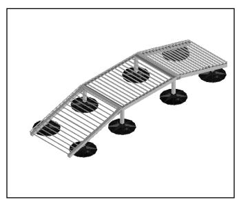
ASP1215R – Crossover Bridge with Ramp – Is designed specifically for use on rooftop without adhesive, roof penetrations, flashings or damage to roofing system. The crossover bridge is utilized for either rooftop or land site application providing an avenue for foot traffic, while protecting cable trays and pipelines. Weight disbursed over 454 sq. in. per support. Custom heights, widths and lengths are available.
